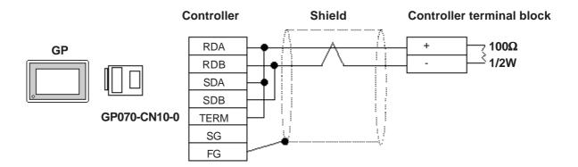
• Using Digital's RS-422 Cable GP230-IS11-0
